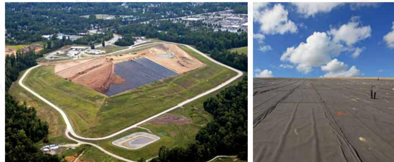
**TerraTextile®** is a specially made technical textile, either woven or non-woven. They offer excellent strength and hydraulic characteristics; and cater for a wide range of applications. **Woven TerraTextile®** is used for soil reinforcement, separation and filtration, secondary reinforcement, erosion control, ground stabilisation, silt fence etc. **Non-woven TerraTextile®** is very popular in applications such as filtration, separation, sub-surface drainage and transmission erosion control.
